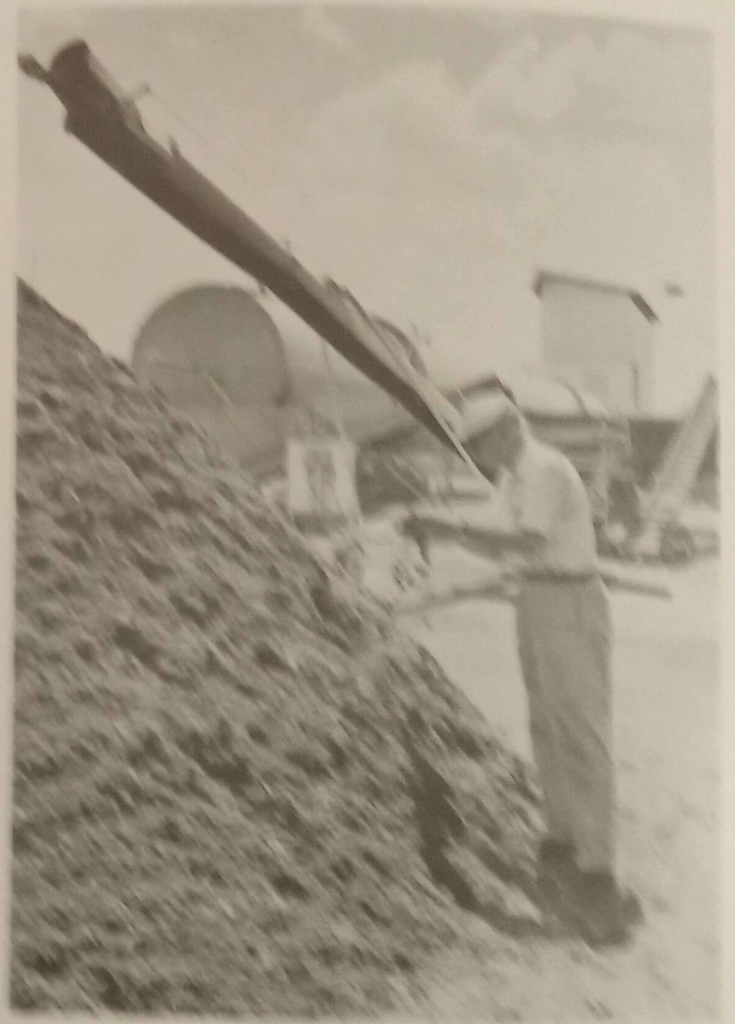
ABOVE: Eric Ewech, inventor, inspects a pile of the final product as it is discharged from the digester, which is pictured in the background. LEFT: Raw garbage is dumped from refuse trucks and pushed into a ramp. A plunger in the ramp forces the wastes into the "big tube." FAR LEFT: An aerial view of the digester site.
